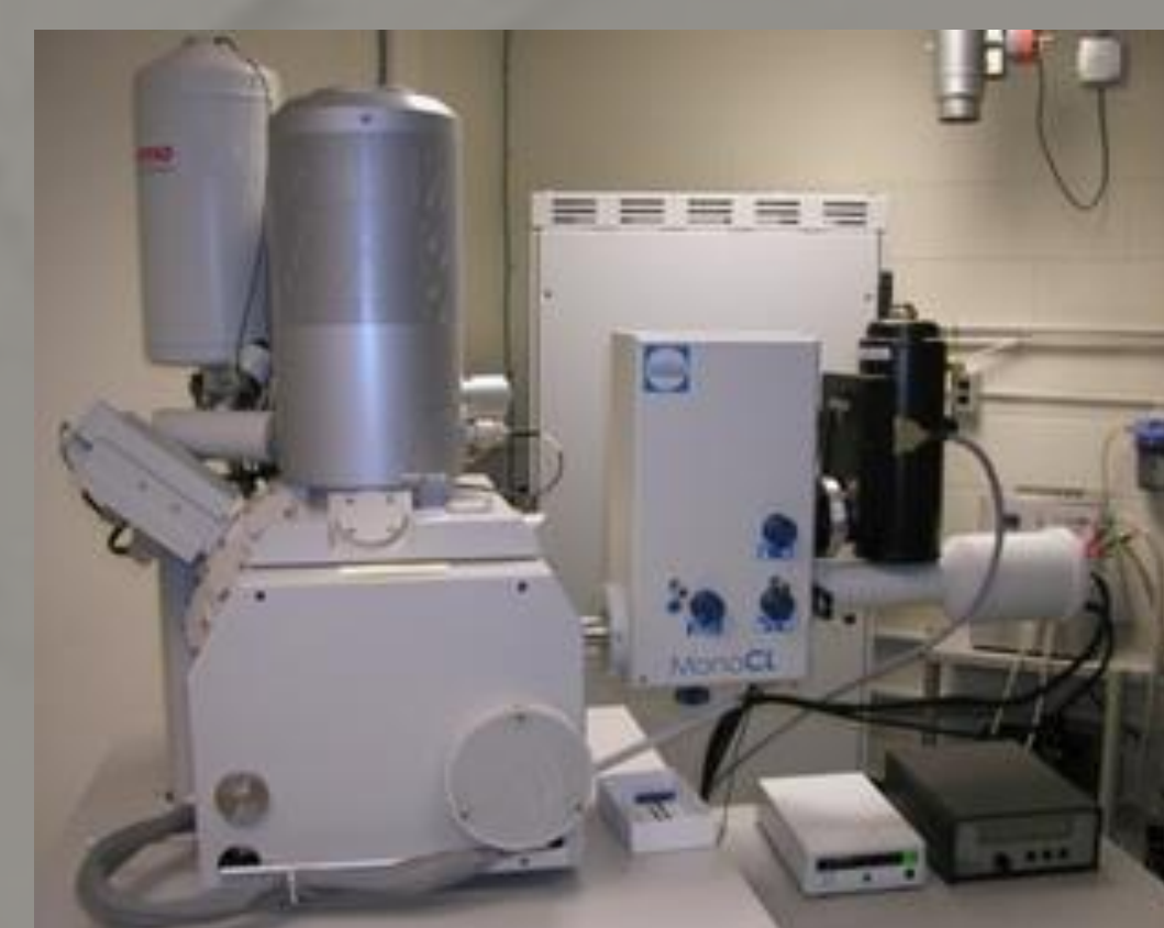
Figure 4. Nova NanoSEM 600 used in study. Image courtesy of http://mineralsciences.si.edu/facilities/sem.htm
