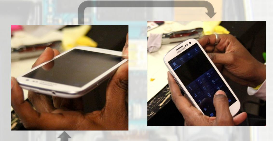
7. Final examination: The technician examines exterior looking for issues with the glass or adhesive. The technician also examines the other functions such as the key board, camera, and power button.
