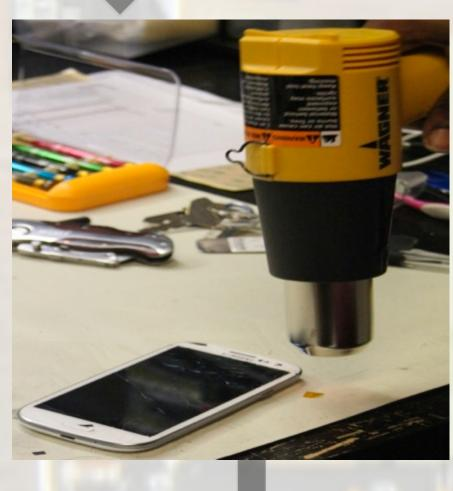
2. Heating up of **Broken Glass:** Technician waves a heat gun over the glass, warming the adhesive behind the glass. Technician repeatedly feels and checks the temperature to avoid damaging the LCD.
