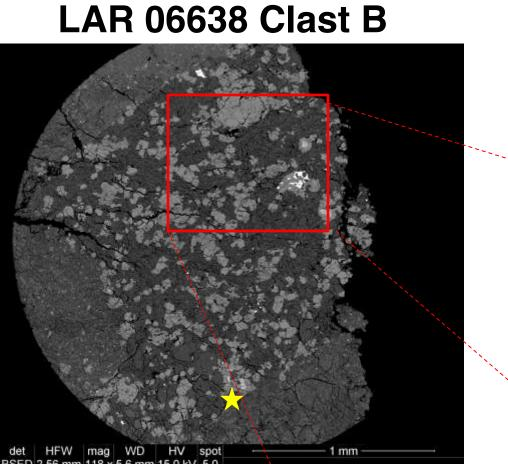
A FEI Nova NanoSEM 600 Variable Pressure Field Emission Scanning Electron Microscope (SEM) was used to closely examine potential basaltic clasts that were located with the Olympus BX61 microscope. The Energy Dispersive Spectrometer (EDS) of the SEM was used to obtain compositional data of individual minerals within clasts.
